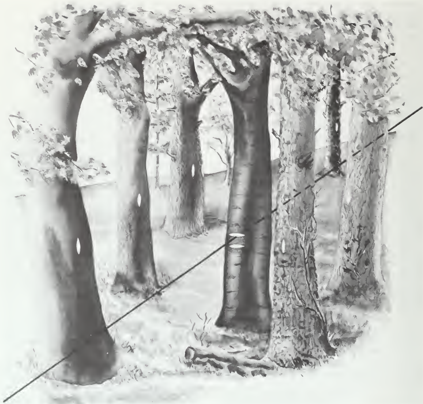
FIGURE 63.—Marking a line through timber.
